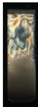
Figure 1. Strong and colorful birefringence in dispersions of Na-Fluorohectorite produced by turbulent flows after shaking.
